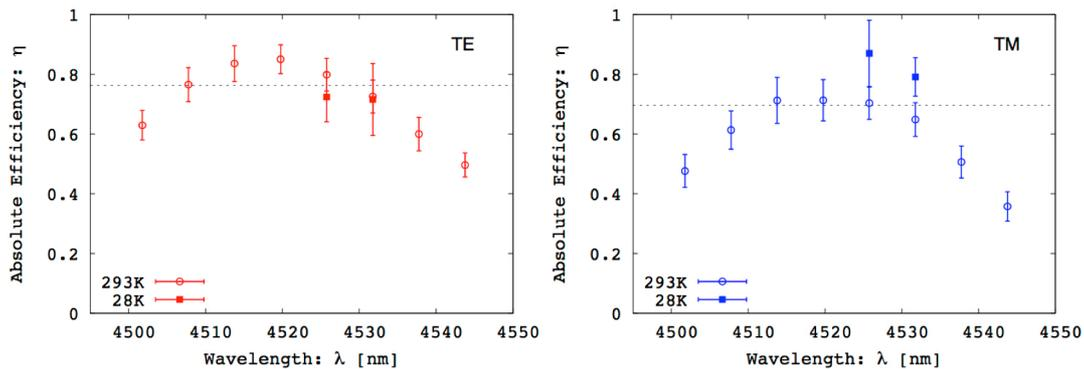
**Figure 4.** Measured absolute diffraction efficiency at room and cryogenic temperatures (left: TE mode, right: TM mode). The horizontal line shows the peak efficiency expected from the design.
