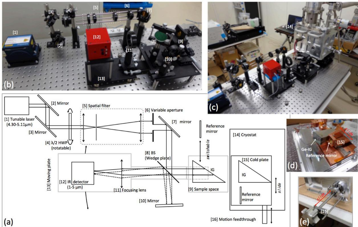
**Figure 3.** An in-house equipment to measure the diffraction efficiency of immersion gratings. (a) Schematic diagram of the optical configuration. (b) Setup for measurement at the room temperature. (c) Setup for measurement at the cryogenic temperature. (d) The Ge immersion grating and the reference mirror on the cold plate. (e) Motion feedthrough.
